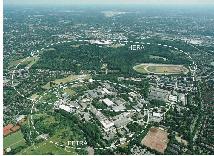
Figure 3.1: The HERA accelerator with the pre-accelerator PETRA. The four circles indicate the different experiments H1, HERMES, ZEUS and HERA-B (clockwise).
